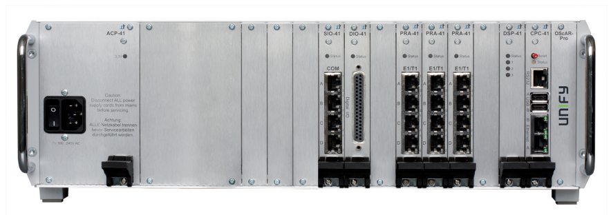
OScAR 300 - Hardware platform of OScAR-Pro 300 V4
